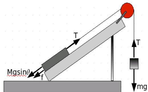
*Illustration 2: Setup to test Newton's second law*
