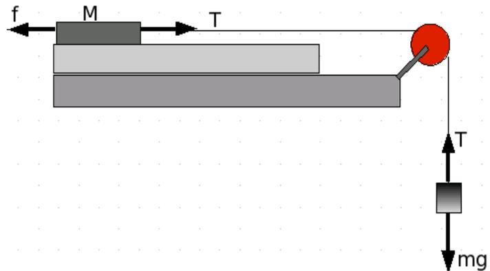
*Illustration 1: Setup to find coefficient of kinetic friction*
